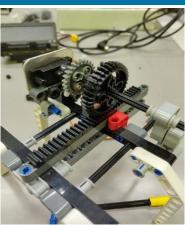
micro servo). Initially the gear caused too much friction thus, a smaller more suitable sized gear was used
