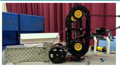
Rubber tracks were placed here these snagged on the claws screws (the claw is attached via screws on the IGUS chain)
