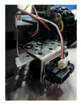
This is how we are able to mount the sensor onto the chassis. The mount as seen on the photo is secured firmly with two nuts and two bolts which would allow for increased stability and overall balance. The sensor will be used to aid in the bot movement.
