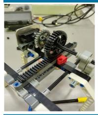
The effector of our robot mainly comprises of a sliding mechanism and a hoist that lift the mechanism itself. This sliding mechanism allows for versatility and efficient multitasking. The effector used here is a claw, as stated before the clay will do many tasks which include lifting supplies and people (also may be used to move other scoring items).
