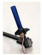
allowed us to create an omnidirectional system, which is better than having the sensor fixed in one place because it allows the robot to sense from any direction and have better functionality for how it is mounted on the robot.
