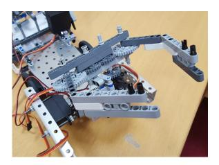
open and close to pick up the poms. We decided a gear system would be the most optimal way to determine the movement of the pincers because of its transmission of torque energy and its ability to control the speed of the movement of the pincers.
