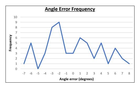
The graph above is a data set we collected for the Angle Error Frequency. The iCreate bot has to make a 90° turn to be in the correct position to grab botguy. We set up a piece of paper underneath the bot, drawing a line at the 90° position that it should turn to. Then we ran the code, and each time the bot completed the turn, we would draw a small line and measure the angle difference using a protractor to see the error.
