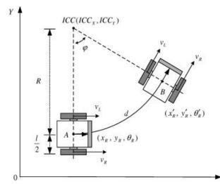
While we can vary the velocity of each wheel, for the robot to perform rolling motion, the robot must rotate about a point that lies along the left and right wheel axis (is collinear). The point that the robot rotates about is known as the Instantaneous Center of Curvature or ICC.
