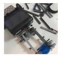
To the left is a picture of the drivetrain. We had initially constructed a chassis from LEGO, but we found that it was difficult to attach the wallaby and motors. As such, we constructed the chassis using a metal base, which we found worked better since the wallaby and motors were held ind the metal base could endure non linear torque much better, therefore both driven wheels would have the same grip at all times. This makes it more reliable and straight line driving more accurate.
