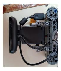
This shows a close-up view of the mount for the camera which will is used to sense for the yellow card placed in front of the burning building. We chose to use the colour sensor for this task because it is the only sensor that will be able to help the robot locate botguy and fema director.
