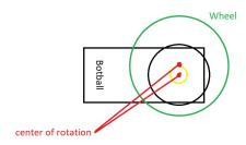
VEX motors have female square hole outputs that accommodate the standard <sup>1</sup>/<sub>8</sub>" shaft size (and <sup>1</sup>/<sub>4</sub>" high strength shaft size on the new V5 motors). As a result, any shafts attached to the motors are concentric and wheels on those shafts are concentric to the motor output as well.
