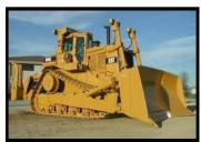
**2.** A Universal Blade ("U-Blade") which is tall and very curved, and has large side wings to carry more material.
