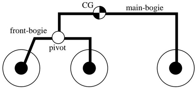
Figure 2: The Rocker-Bogie Mobility System
