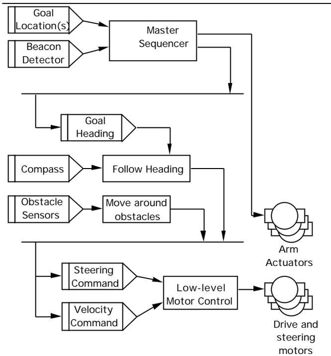
Figure 6: The Structure of the Control Software
